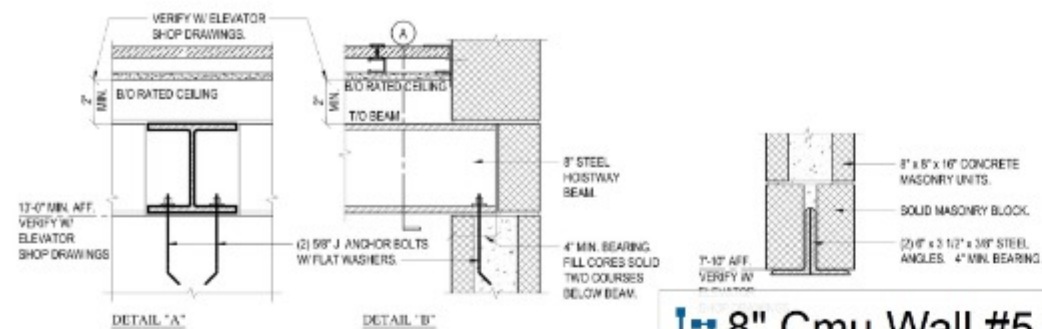
11 HOISTWAY BEAM BRACING DETAILS SCALE: 1/2" = 1'-0"
