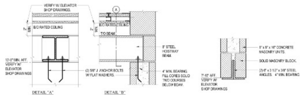
11 HOISTWAY BEAM BRACING DETAILS SCALE: 1/2" = 1'-0"
